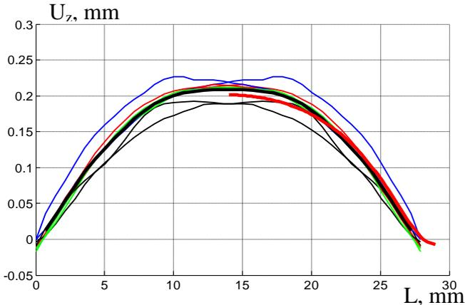
Figure 2: Relative residual axial displacements on the cylinder upper face
